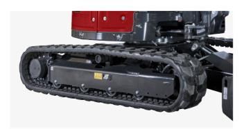
The X-shaped box-section structure of the undercarriage provides excellent torsional stiffness. The frame is designed for maximum durability.
