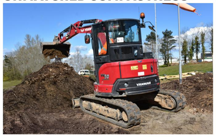
The ViO50-6B is providing Yanmar customers with true peace of mind, especially in urban environment where space is limited. The new design of the ViO50-6B boom also offers a very compact turning radius.
