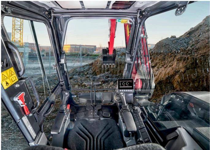
The SV86-7's cabin is meticulously crafted to cater to the driver's needs. Its ergonomic design offers a comfortable and intuitively organized workspace, optimizing productivity throughout extended days at the construction site. Exceptional all-around visibility and thoughtful design elements ensure a fatigue-free work environment, prioritizing both comfort and safety for maximum operational efficiency.
