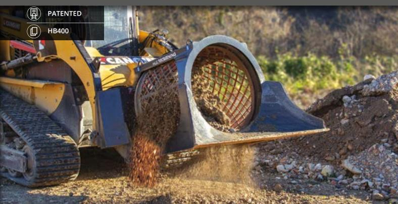
THE NEW MULTISCREENING BUCKET WITH THE NEW ROTARY DOUBLE DRUM CONCEPT FOR FRONTAL COUPLING AND MACHINES UP TO 14 TONS (30865 LB) IS SUITABLE FOR SELECTION DUTIES ON TURNED SOILS AND RESULTING MATERIALS. THE MATERIAL SIZE CHANGE – FROM 25 TO 60 MM (1 - 2,4 IN). - IS CONTROLLED DIRECTLY AND HYDRAULICALLY FROM THE CAB WITHOUT REPLACING ANY MECHANICAL PART THUS REDUCING THE WORK TIMES CONSIDERABLY.
